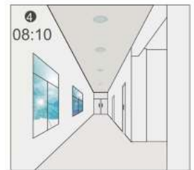
4 08:10 When the natural light level exceeds setpoint off to light, the light will turn off even if when the space is occupied.
