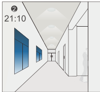
The light dims to 50% waiting level after the hold-time.
